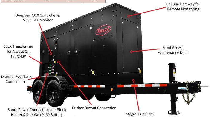
$\textbf{General Guidelines for Deration:} \ A lititude: Derate 0.5\% \ per 100m (328 \ ft.) \ Elevation above 1000m (3279 \ ft.) \ Temperature: Derate 1.0\% \ per 10^{\circ}C (18^{\circ}F) \ temperature above 25^{\circ}C (77^{\circ}F) \ temperature above 25^{\circ}C (77^{\circ}C) \ tempera$
